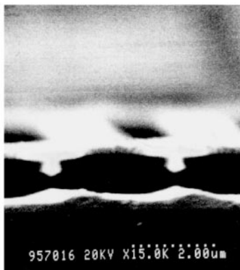
Fig. 1. a Schematic of pentagon-shaped silicon wires. b Cross-sectional SEM image of as-etched pentagon-shaped silicon nanowires prepared by the selective etching
